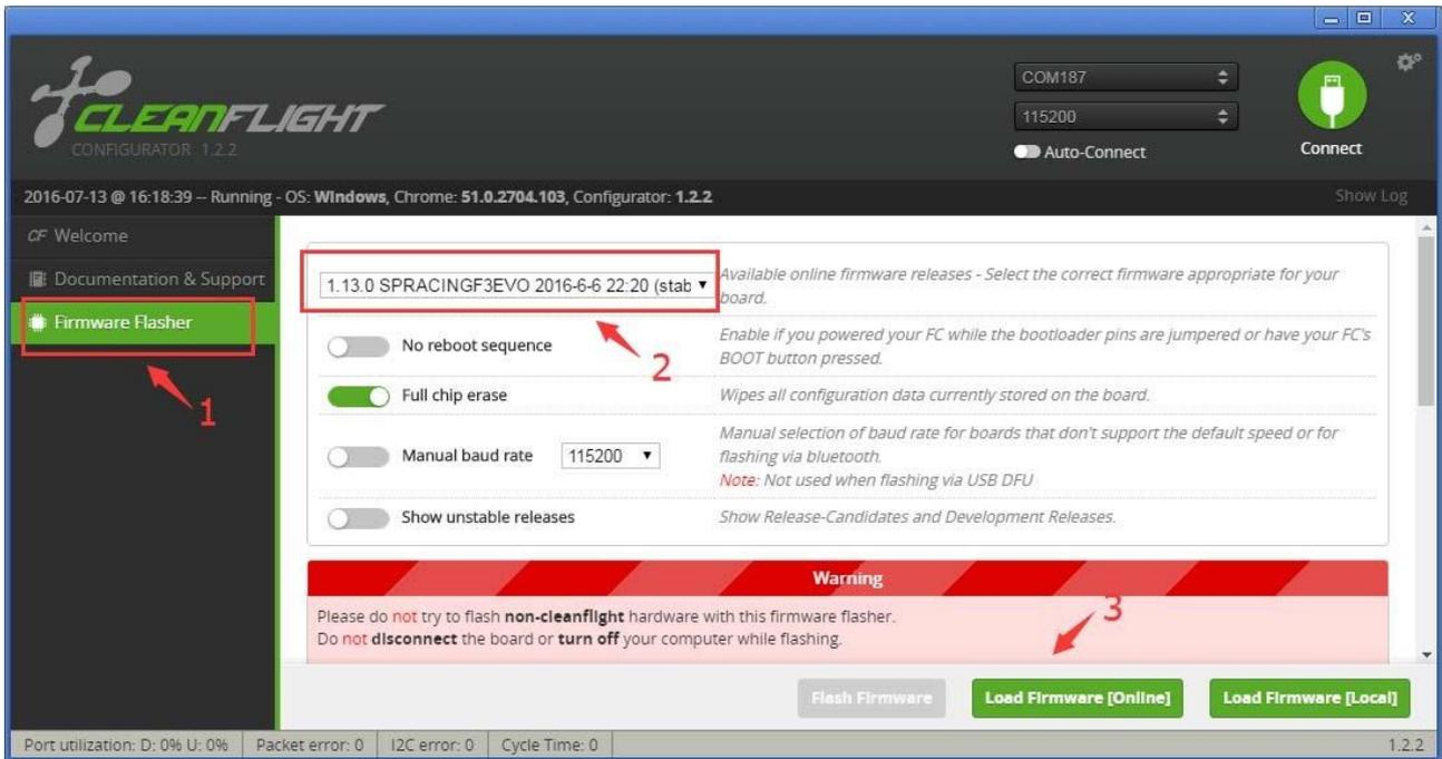
3. Click "Flash Firmware" and wait the ST DFU DRIVER Automatic installation. It's successfully installed when you see the DFU port on the Up right corner.
