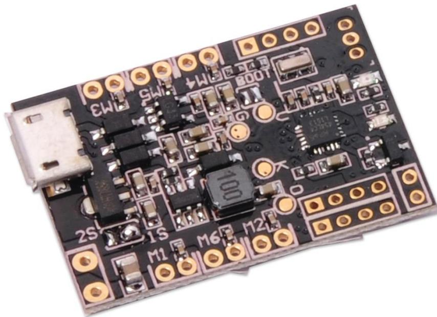
**The Hyperion F3 EVO Brushed Flight Controller gives you all the features in a small size and designed for micro size quads with brushed motors. Supports up to 6 motors for Hex copter configurations.**
